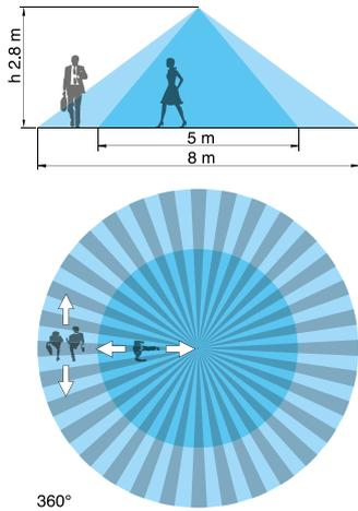
18.31...0031 - Internal ceiling installation, surface mounting
