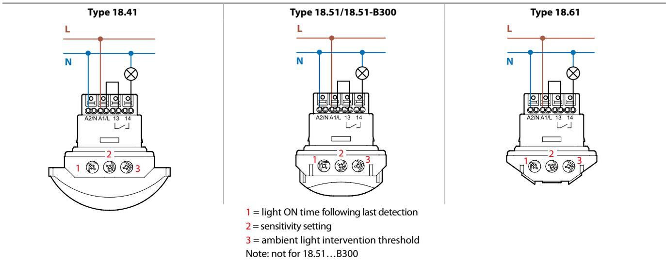
The nominal lamp rating as stated in the contact specification applies when wiring is realized in accordance with the diagrams above. If the load is powered from a phase different to that powering the Movement detector, then a 50% reduction in the lamp rating must be considered.
