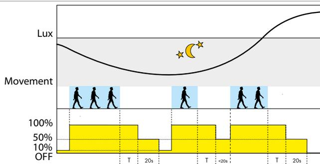
**Courtesy - ON/OFF control with early warning + courtesy light level**
